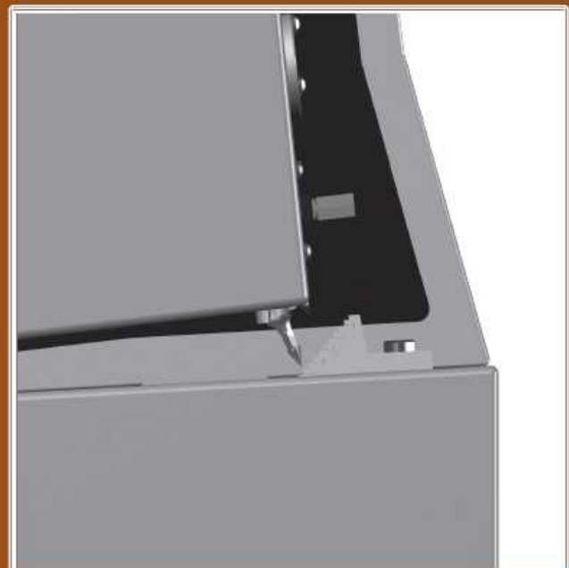
FIGURE 10 - POSITION REAR SPIKE OF THE LOWER TWEETER/MIDRANGE MODULE INTO THE PROPER BLOCK STEP
