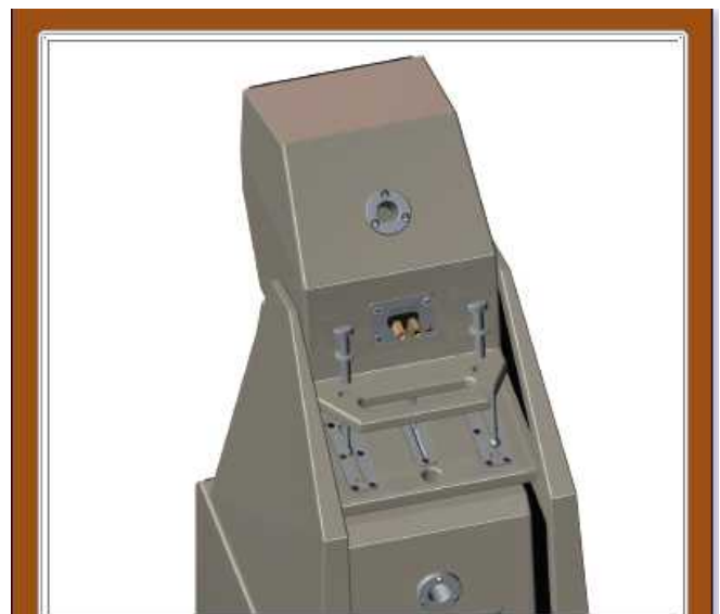
FIGURE 14 - INSTALL THE TETHER BOLTS IN UPPER MODULE
